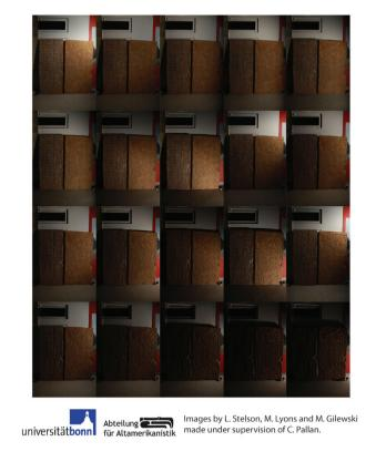
**Figure 2.** 20 (of 68 total) digital images (with various light direction) taken to produce the RTI image shown in Figure 1.
